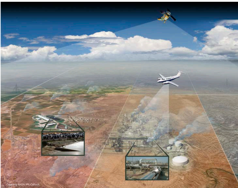
Illustration of a tiered approach to methane measurement, combining satellites, airplanes, and ground-based sensors. Figure courtesy Riley Duren, NASA/JPL-Caltech
