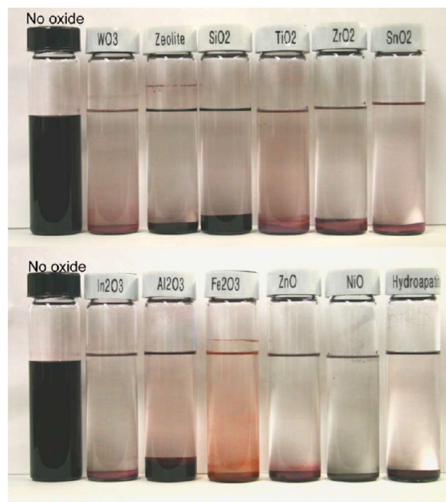
Figure 3. Deposition of 6.3 nm Au nanocrystals capped with dodecanethiol (vials on the left) on several oxide supports in chloroform. The powders settle at the bottom of each vial leaving a colorless supernatant and indicating a complete deposition of the nanocrystals on the support surface. The nature of the solvent is crucial for a successful deposition. Reprinted with permission from ref 50. Copyright 2006 American Chemical Society.
